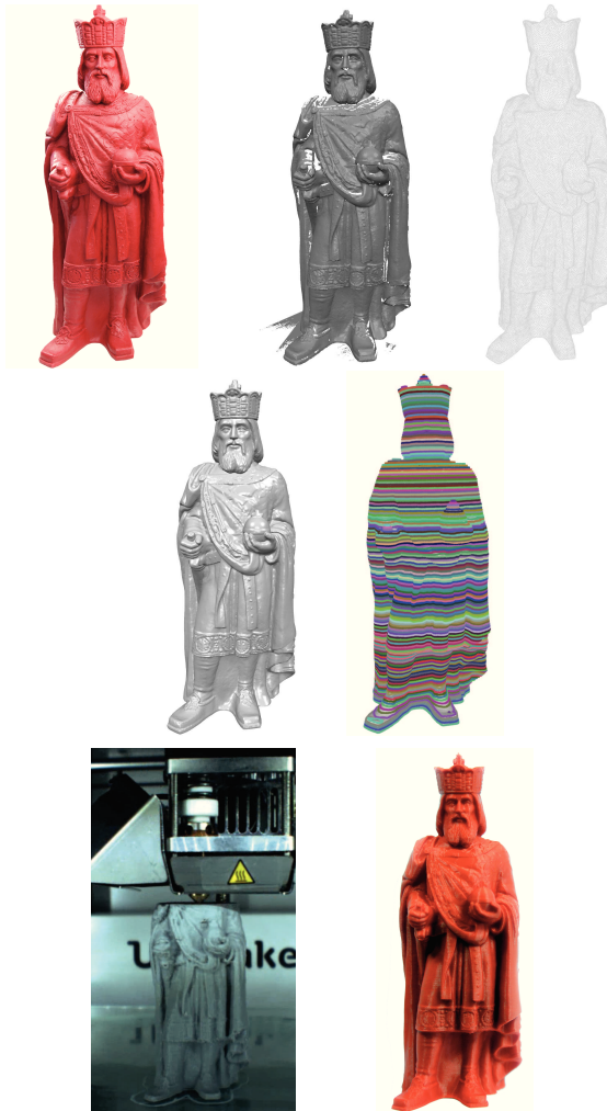
Figure 2.7: 3D printing pipeline: Original model, scanned model with holes, remeshed model in wireframe and shaded, sliced model, printing, printed model.
