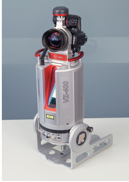
Figure 2.3: Riegl VZ-400 long-range laser scanner with Nikon D800 with 14mm ultra-wide lens mounted on top.
