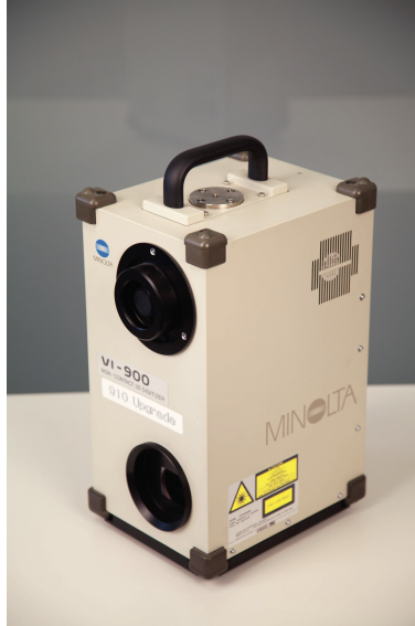
Figure 2.1: Minolta VI-900 laser scanner. Top opening contains the camera. Bottom opening encloses a laser emitter.
