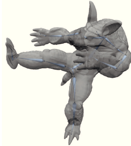
Figure 2.9: Screenshot of a 3D surface mesh of an Armadillo with an attached skeleton inside it. The surface can be deformed by moving the skeleton in its interior.
