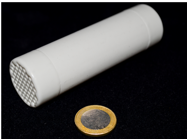
Figure 3.2: Ceramic membrane monolith comprising 55 feed channels
