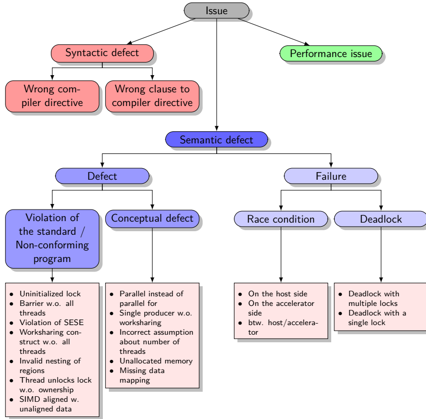
Figure 5.2.: Classification of common issues in OpenMP applications [65, 22].
