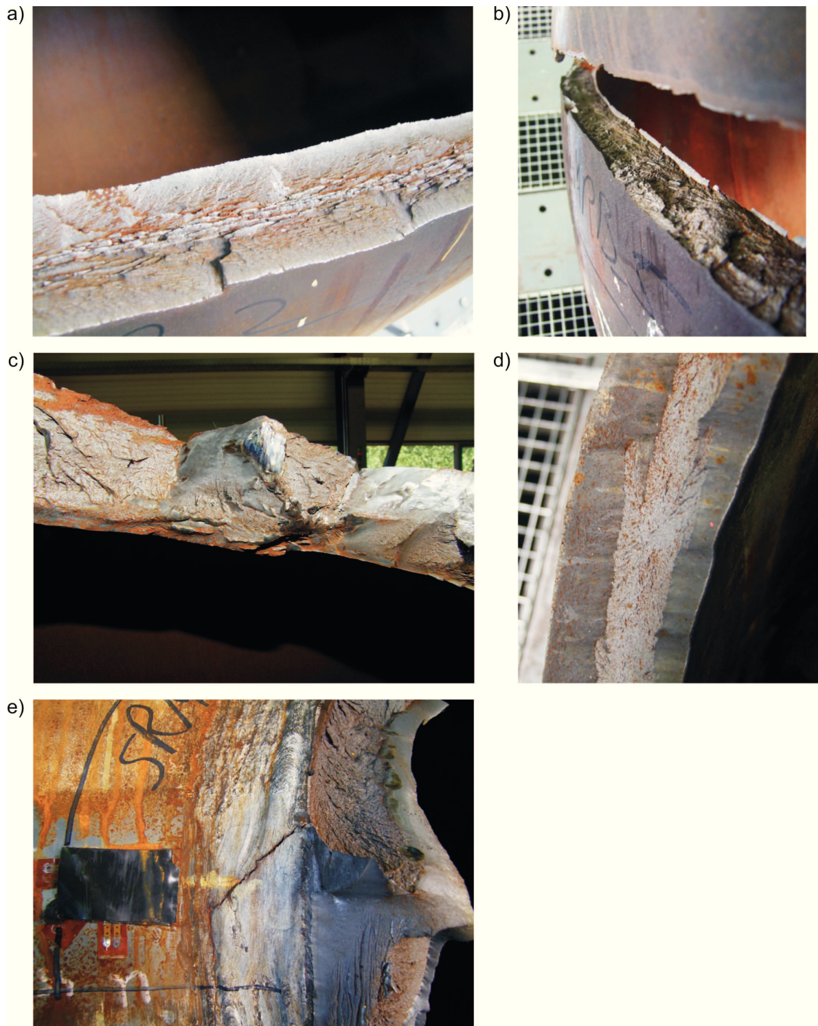
Figure 7.33.: Details of typical fracture surfaces in: a) dvII-body, b) dvIII, c) dvIV d) dvII-nozzle and e) detail of a small crack on the weld seam.
