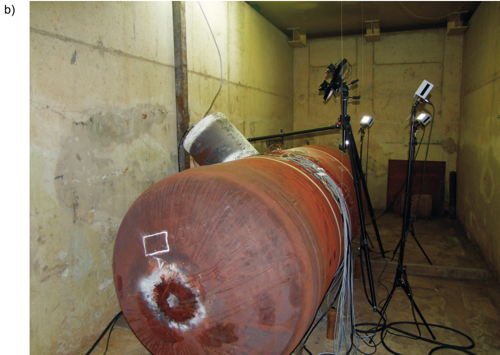
Figure 7.7.: a) Schematic illustration of the vessel instrumentation. b) The instrumented vessel in the burst cavern.
