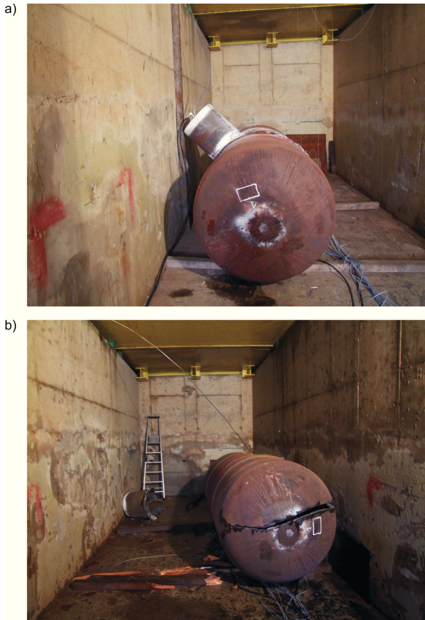
Figure 7.28.: The pressure vessel in the burst cavern a) before and b) after the burst test.
