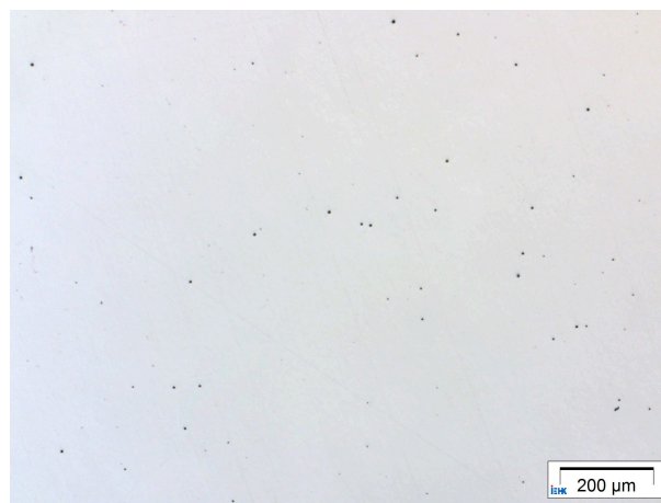
Figure 7.12.: Polished section of dvII for the determination of the inclusion content at a magnification of 100.
