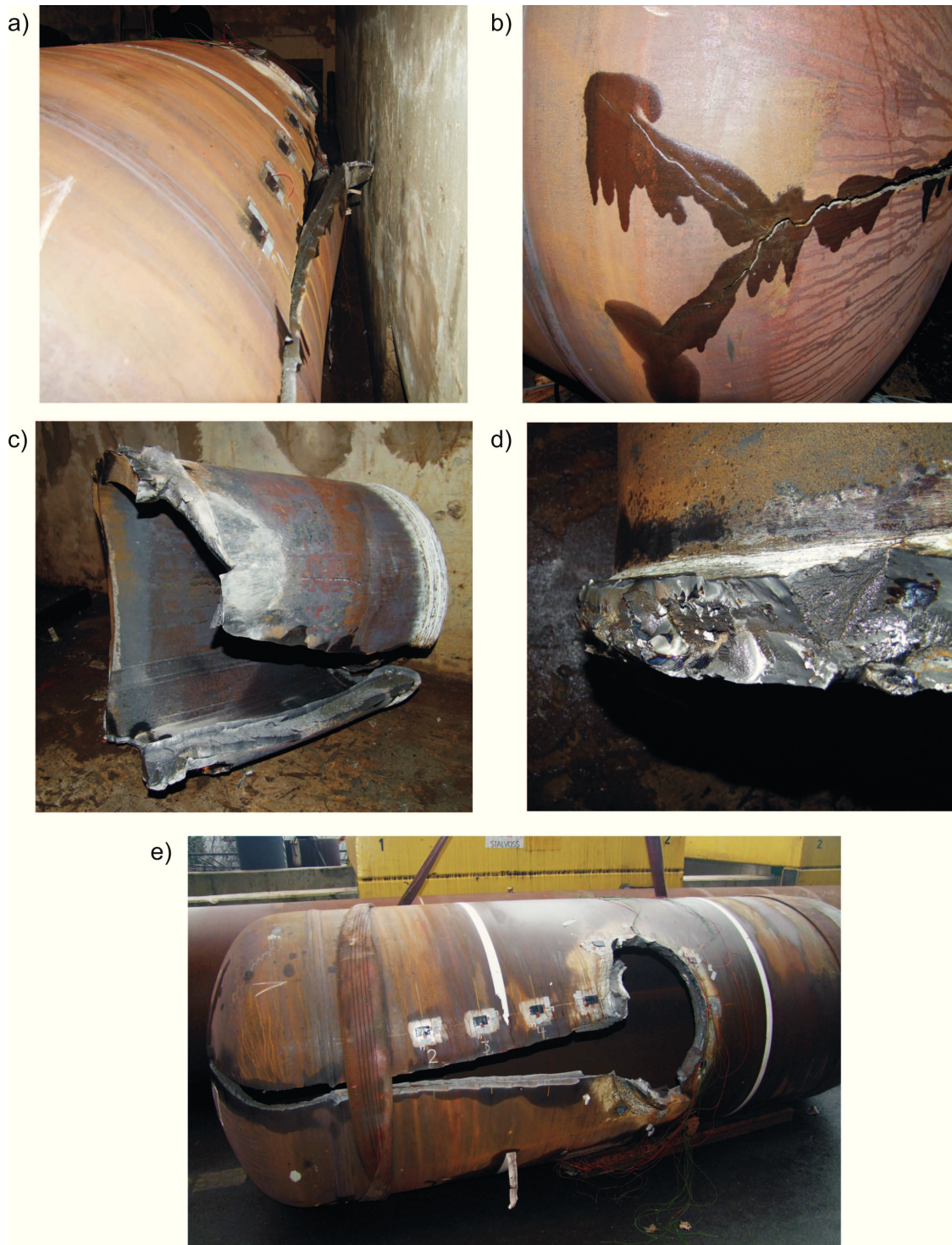
Figure 7.29.: Details of the crack path: a) Crack in the vessel body, b) split end of crack in the front heading, c) split nozzle d) heat tinted material at the nozzle crack surface, e) crack path in the vessel body, visible after relocation from the burst cavern.
