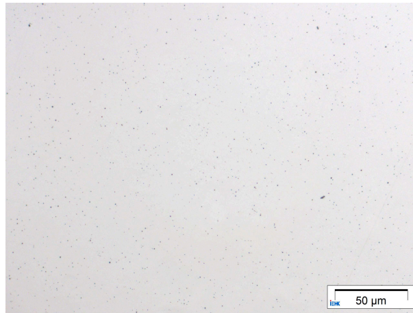
Figure 7.19.: Polished section of dvIV for the determination of the inclusion content at a magnification of 500.
