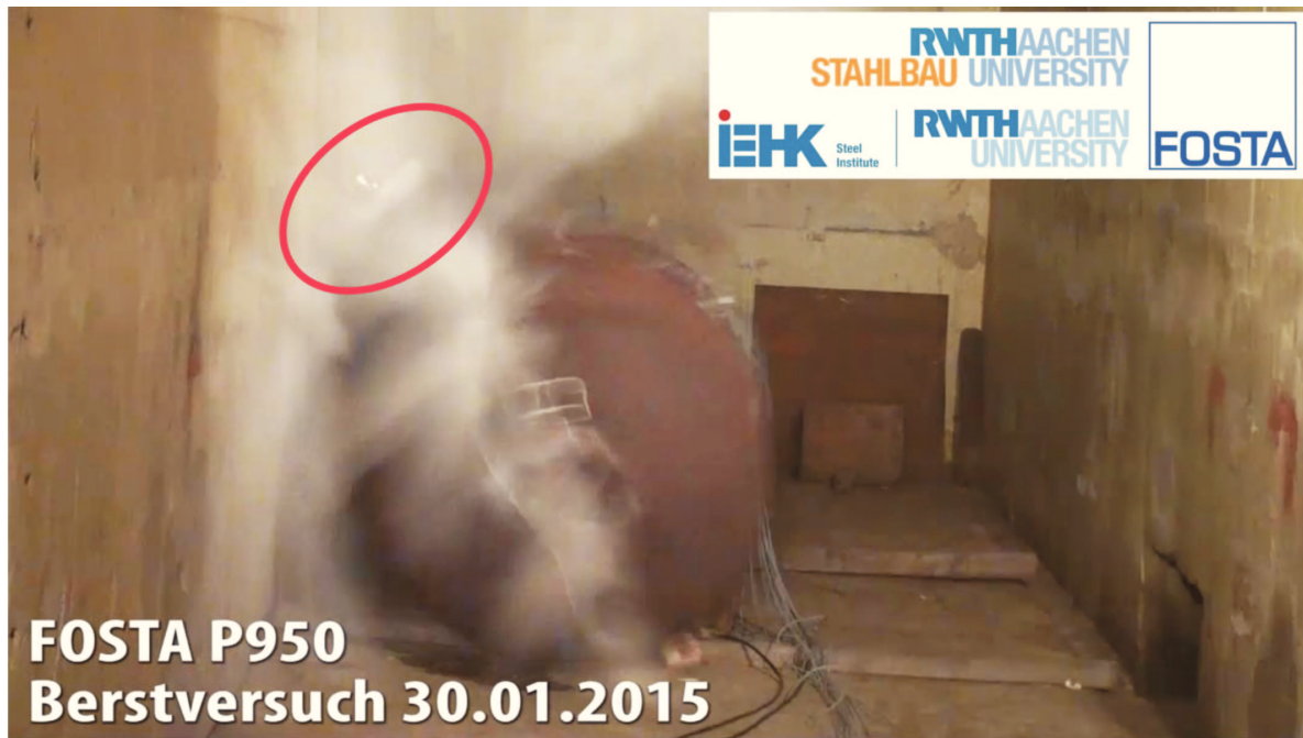
Figure 7.35.: Last frame of the test video in which the vessel is recognisable. The crack in the head is already visible while the nozzle, recognisable by the white paint on its top and marked by a red circle, is still in its place and uncracked.
