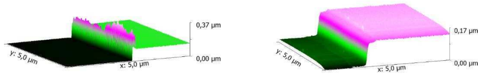
Figure 4.6 AFM graphs of the bottom electrode (TiN / Ti / Au / Cr / Sapphire): without collimator (left), with collimator (right).
