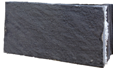
Figure 7.6: Aluminium plate coated with high temperature resistance glue mixed and dried with one layer of JSC-2A lunar regolith simulant. Image 90°rotated.
