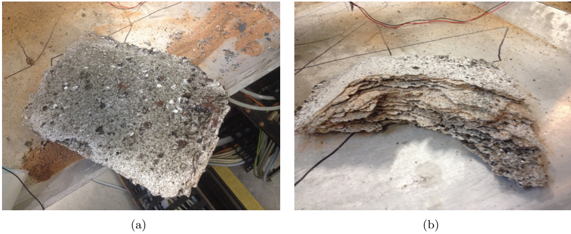
Figure 8.2: Solar sintered block of sand (a) and a cross-section of the same part (b).
