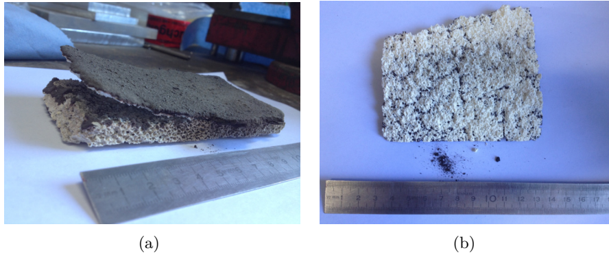
Figure 7.4: (a) Thermal stresses breaking the porous ceramic substrate. (b) Sintered part in contact with the substrate.
