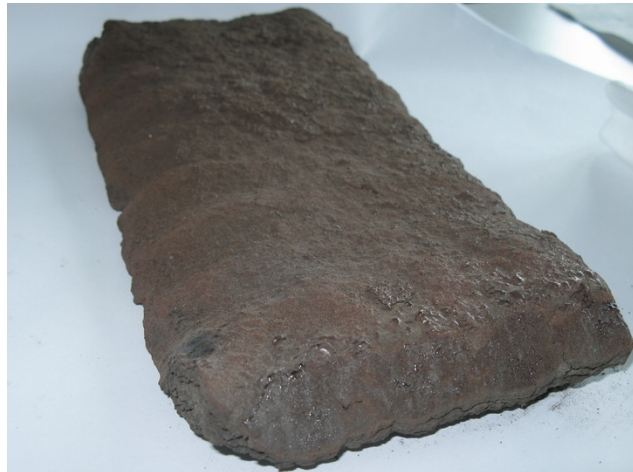
Figure 5.18: Brick obtained using Test 4 parameters. The substrate and the top layer, created after the 7-minute stop, were removed.
