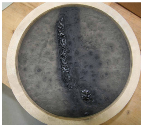
Figure 4.2: Fresnel lens combined with a rover and a mirror (left) and regolith testbed with solar sintered material (right) [82].
