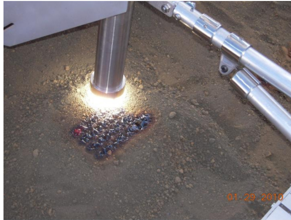
Figure 4.1: Sintered regolith simulant by concentrated solar light into an optical fibre, [83].
