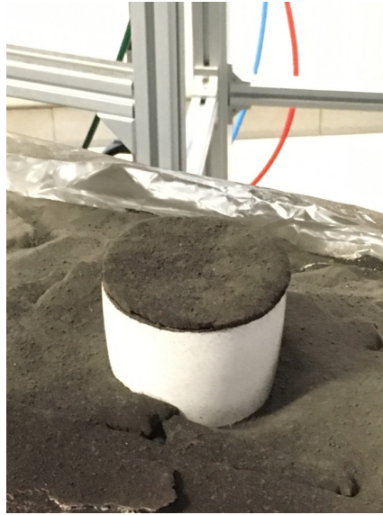
Figure 5.29: Sintered regolith with Test 11 parameters at the end of the process.
