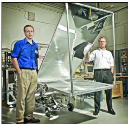
Figure 4.2: Fresnel lens combined with a rover and a mirror (left) and regolith testbed with solar sintered material (right) [82].
