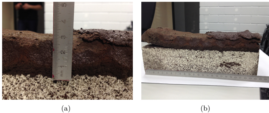
Figure 7.3: Brick solar sintered on a porous ceramic substrate using Test 4 parameters (a). The regolith bonded with the porous ceramic substrate (b).
