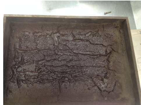
Figure 5.5: Typical sintered plane of JSC-2A lunar regolith simulant where sintered lines are too close to each other. Dimensions of the testbed: 270 mm x 200 mm.
