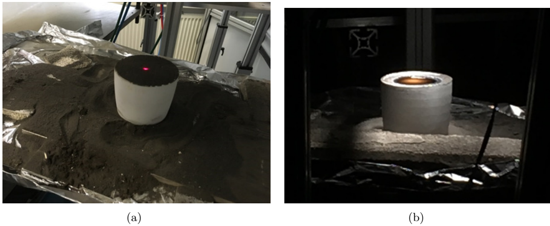
Figure 5.28: Crucible filled with lunar regolith simulant before (a) and during (b) melting.
