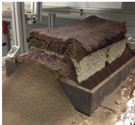
Figure 5.16: Brick obtained using Test 4 parameters. The picture was taken right after the end of the process.
