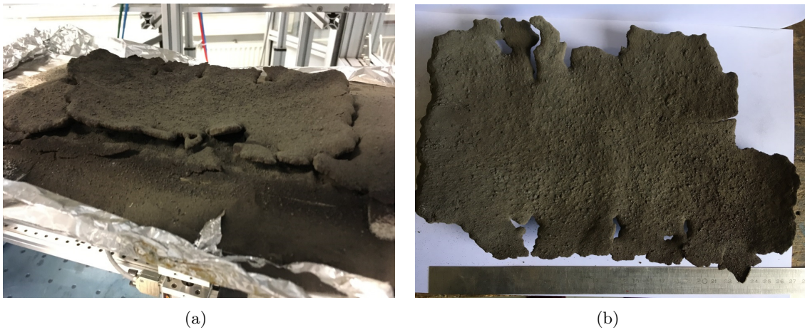
Figure 5.25: Solar sintered part after a 2-hour process and Test 8 parameters: side (a) and top (b) views.
