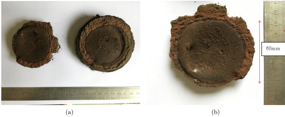
Figure 5.32: The molten part was detached from the sintered one (a). The top side, which was in contact with the sintered regolith simulant, showed a tiny amounts of sintered grains connected to it, proving the poor bonding between melt and sintered regolith (b).
