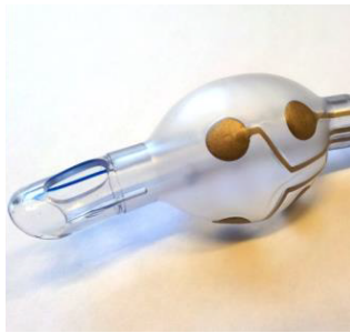
Figure 3: Endotracheal tube with integrated electrodes on the cuff used throughout this study.
