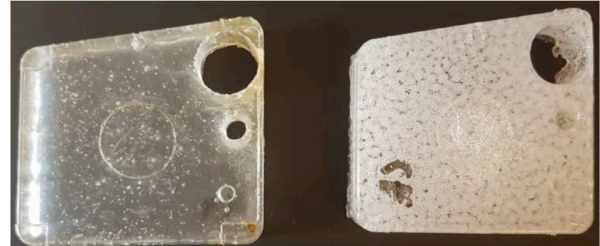
Figure 4: Cured jig made from TOPAS granulate (left) and CALIBRE granulate (right)
