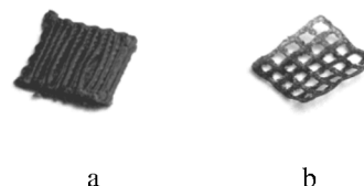
Figure 2: 3D nanocomposite bioconstructions obtained from a grid trajectory with a distance of 0.5 mm (a) and 1.5 mm (b) between parallel lines
