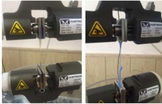
Figure 3: Stretching test of gelatin (left) and silicone (right) samples.
