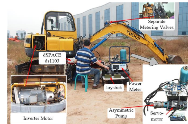
Fig.5 Photograph of mini-excavator with the proposed system
