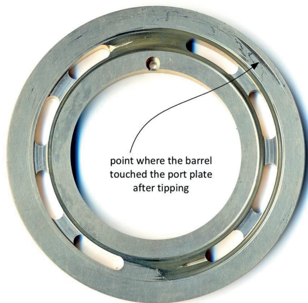
Fig. 5: Port plate showing the tipping mark of the barrel
