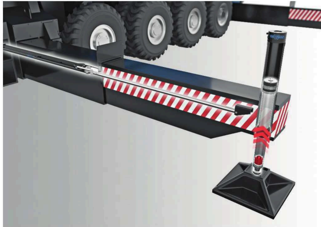
Figure 2: Supporting cylinder with integrated force measurement
