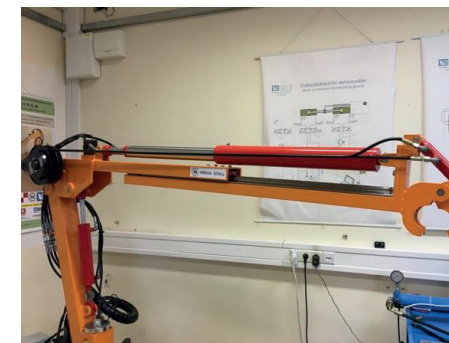
Figure 5. Telescopic hydraulic cylinder used for the linear movement of the extendable arm
