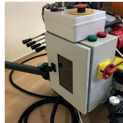
Figure 11. Designed and manufactured wireless control assembly
