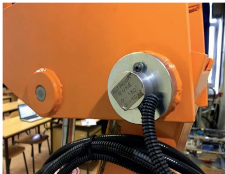
Figure 9. Rotary encoder for measuring telescopic arm rotation
