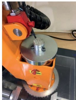
Figure 8. Rotary encoder for measuring base rotation
