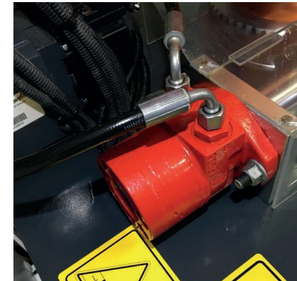
Figure 3. Hydraulic torque motor paired with a worm drive
