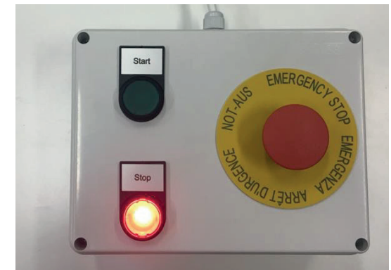
Figure 156. Control box for the additional safety in turning the system on and off
