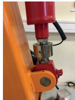
Figure 10. Force sensor for measuring payload
