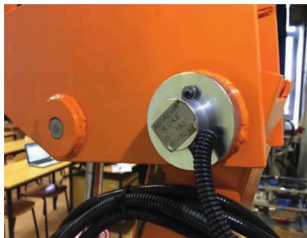
Figure 9. Rotary encoder for measuring telescopic arm rotation
