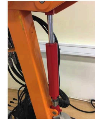
Figure 4. Double acting hydraulic cylinder used for the rotation of the telescopic arm
