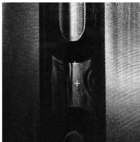
Figure 5. Combined Raman spectroscopy and Mach-Zehnder holography: distance between the measuring points (lowest point of bubble and laser spot) where the concentration was measured. Reproduced from ref. [23]
