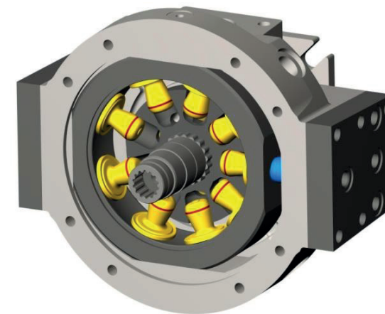
Figure 3: RAC principle: Radial pump with axial portplates
