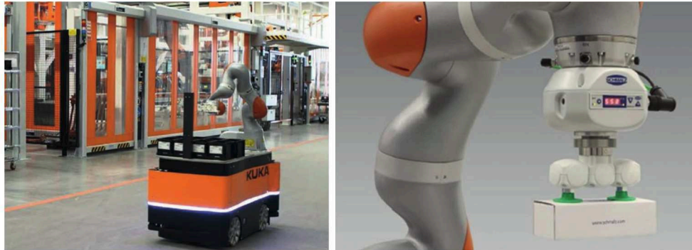
Figure 6: Mobile platform with robot (left – source: KUKA Aktiengesellschaft), Schmalz-CobotPump – electrical vacuum generator for CoBots (right)
