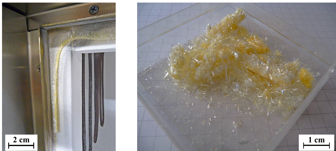
Figure 3.18 Evaporated flux material found on the door of the furnace (left). The crystals form opaque and yellow aggregates (right). Single crystals are transparent and have a pearly lustre. Their size is about 2 mm by 5 mm while being very thin ( < 1 mm).
