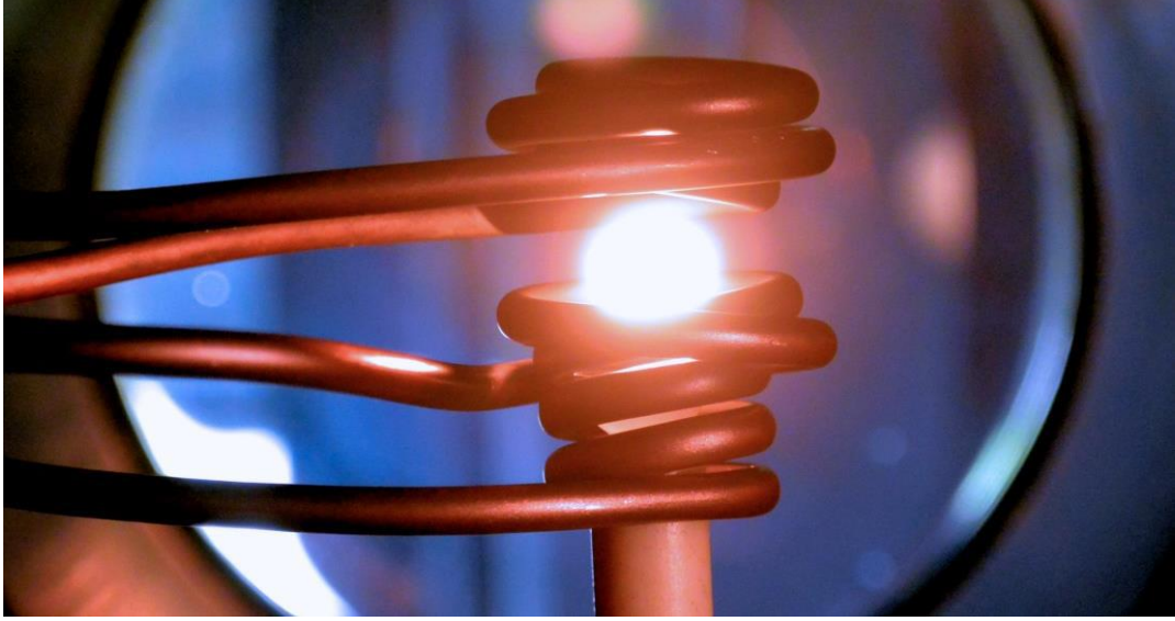
Figure 3.1: Photograph of an electromagnetically levitated liquid iron sample at a temperature of about 1873 K. Copyrights granted by C. Karrasch and taken from reference [70] Fig. 4.1.
