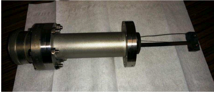
Figure 3.16: Picture of the titanium sublimation pump used at the DLR-MP.
