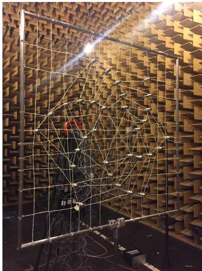
Figure 3.11.: The spiral microphone array used in the measurement.
