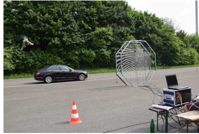
(b) Car02 pass-by measurement.
