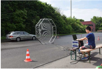
(a) Car01 pass-by measurement.
