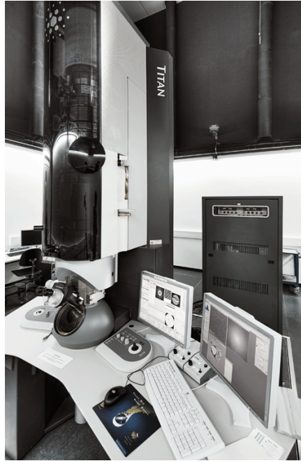
Figure 1.1.: Picture of the FEI Titan G2 60-300 HOLO, installed in the Ernst Ruska-Centre for Microscopy and Spectroscopy with Electrons (ER-C) in the Jülich research centre. This fourth generation TEM is optimised for the investigation of electromagnetic fields in materials using off-axis electron holography. Image taken from [44].
