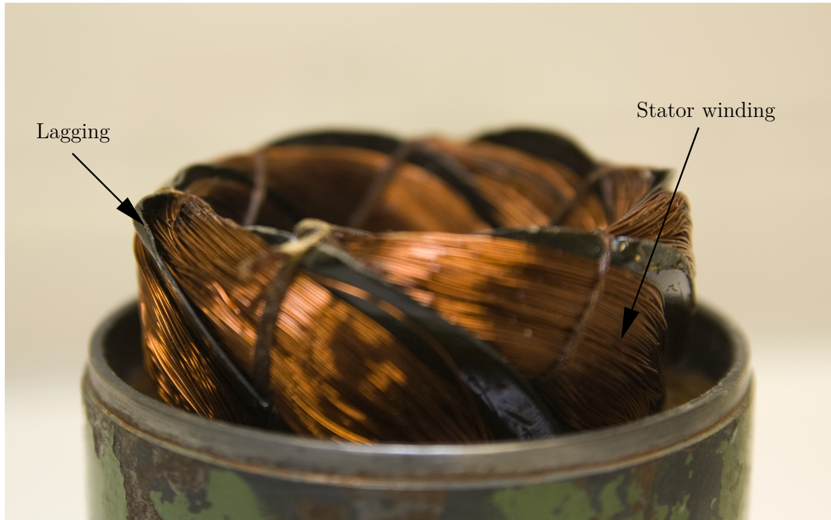
Figure 4.9: Stator winding and the lagging
