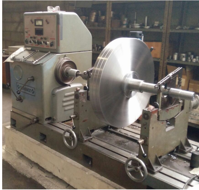
Figure 4.19: Balancing of the flywheels and the shaft on a Schenck balancing machine (thanks to Thouet GmbH)
