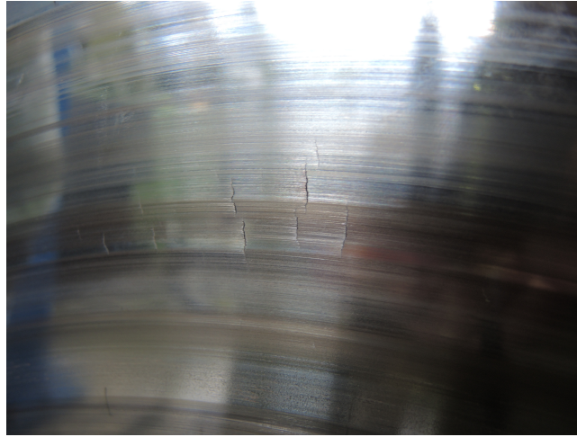
Figure 1.3: Haircracks on the friction surface of a brake disc of a high speed train (Acknowledgement to the IFAS for the good cooperation)
