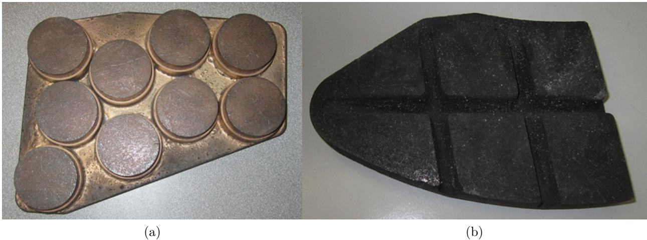
Figure 1.1: (a) One half of a sintered brake pad of a train, (b) One half of an organic brake pad of a train
