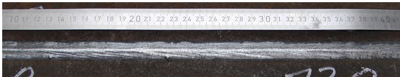
FIG. 12. SA-LAHW weld upper bead: D_{LA} = 14 mm; welding travel speed 0.6 m/min; laser beam power 16 kW.
