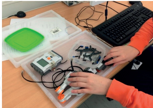
Figure 3. Prepared Lego Mindstorm system for students who are blind.
