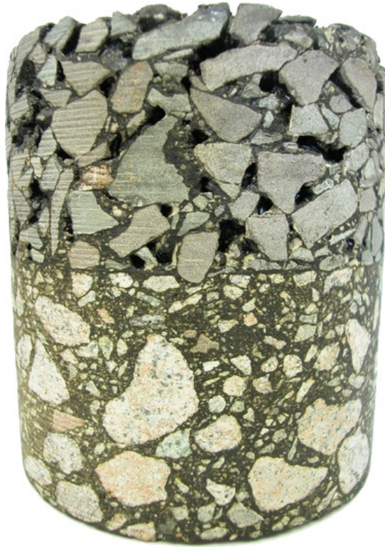
Figure 1.1: Drill core with two different types of asphalt. The top layer is an open-porous asphalt, whereas the bottom layer is dense. Published under CC-BY-SA-3.0 as "Core porous asphalt" by VBW-Asfalt, cropped from original.
