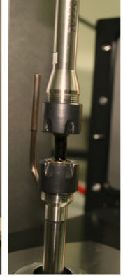
Figure 3.3: Left: Overview of the rheometer setup. Right: Closeup of the specimen in the testing device.
