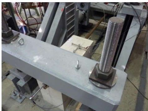
Figure 3-2 Photograph of beam-end test setup (left) and test specimen drawing with reaction plate dimensions (right)
