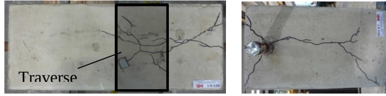
Figure 3-12 Crack formation at top (left) and front side (right) in beam-end test BET-9-1 with transverse pressure
