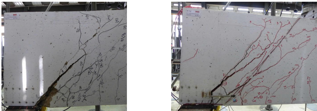
Figure 3-55 Crack pattern in test V1-1 without induced crack (left) and test V1-2 with induced crack (right) after failure
