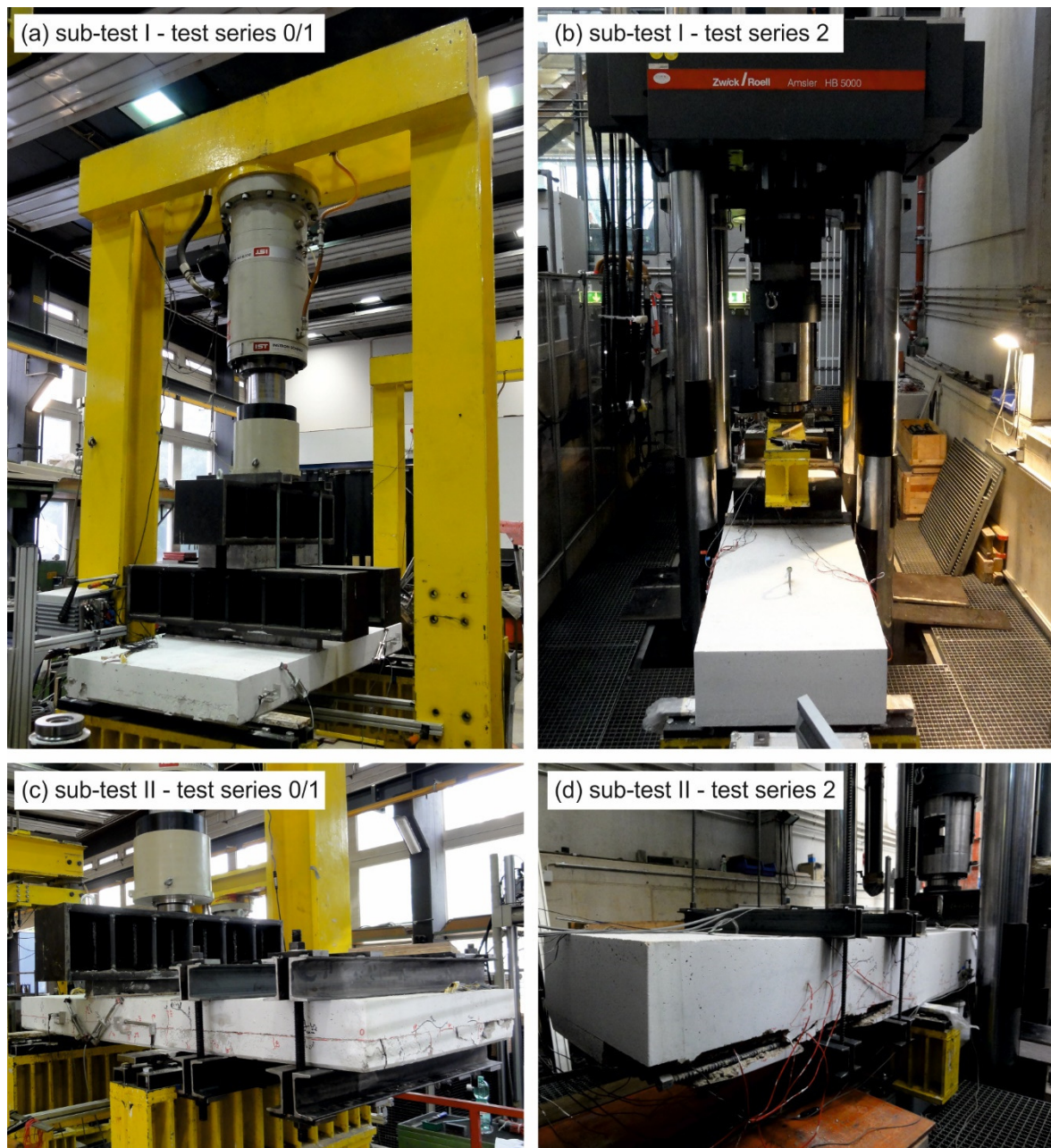
Figure 5-15: Test setup for fatigue tests: sub-test I for test series 0/1 (a), sub-test I for test series 2 (b), sub-test II for test series 0/1 (c), sub-test II for test series 2 (d)
