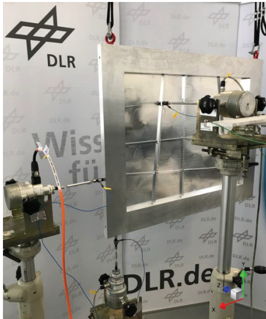
Figure 7: Aluminum plate configuration for Force control
