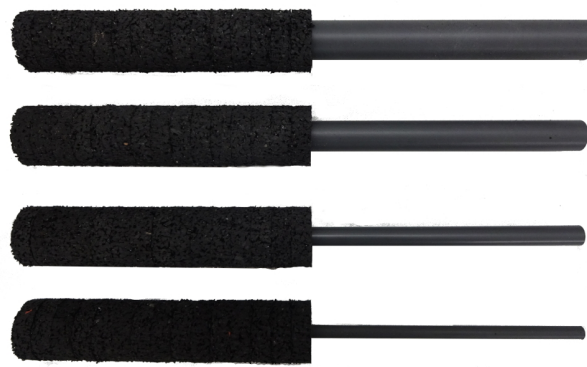
Figure 1. Photograph of the four cylinders (half-)covered by Damtec Black Rubber (from top to bottom: d = 20 mm, 15 mm, 10 mm and 6 mm)
