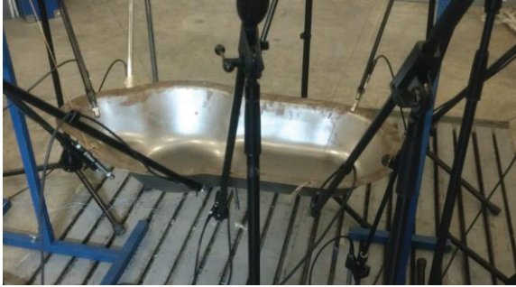
Figure 3 - Oil-pan setup in semi-anechoic room.
