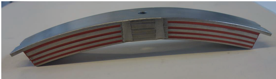
Figure 2 – This is a wheel absorber for radial damping
