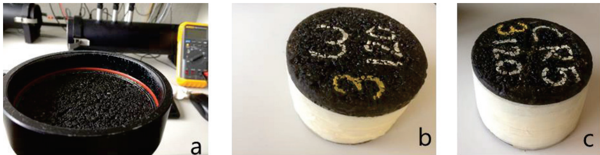
Figure 3 Specimens used for acoustic tests a)Dense asphalt, b)SDA4 Pmb, c)SDA4 CR
