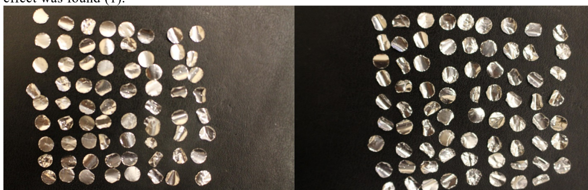
Figure 2 Aluminum foil discs sonicated by 33 sec in the beaker reactor. (a) Freely dropped (b) In container.
