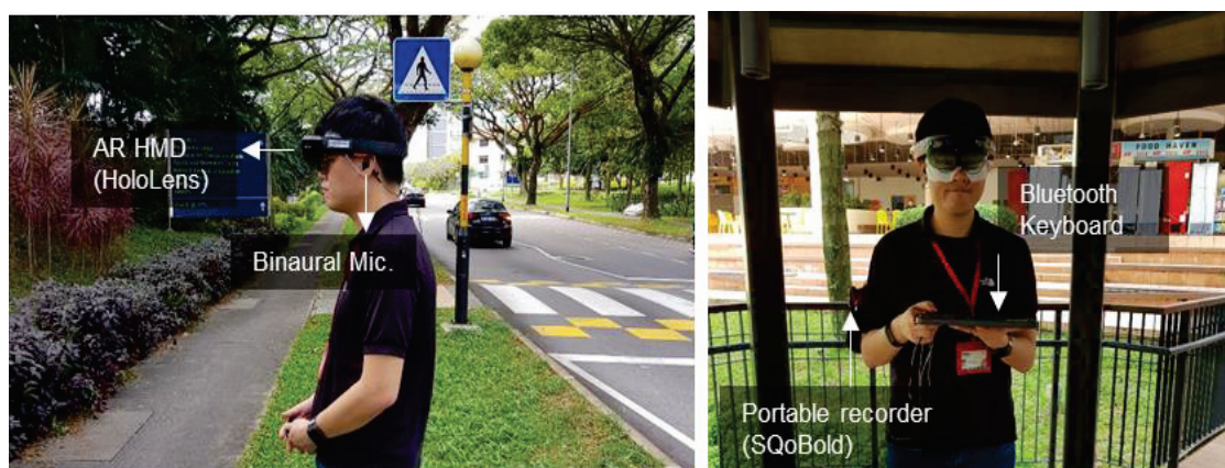
Figure 2 – Equipment setup for the in situ AR experiment
