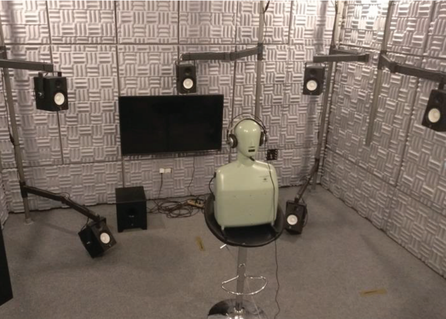
Figure 5 – Calibration of the system with the headphones on the dummy head
