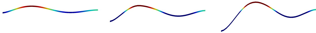
Figure 3. 1500Hz excitation frequency, vibration pattern for the the starting guess (left), optimized design with 1 element in the vertical direction (middle) and optimized design with 5 elements in the vertical direction (right).
