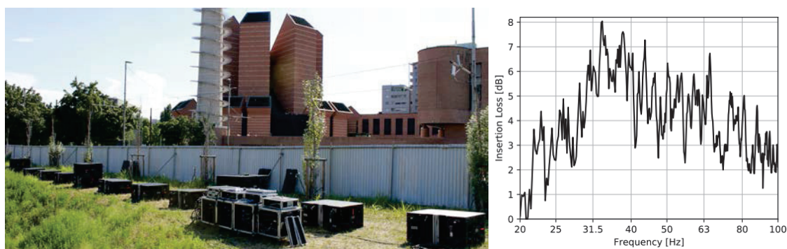
Figure 5 – The full-scale pilot test at Kappa FuturFestival. Left: In the foreground the 20 subwoofer secondary array. In the background is the church building that was used as the dark zone. Right: Estimated average Insertion Loss, from [3].
