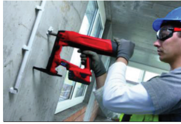
Figure 10 – The battery-driven fastening tool is capable of fastening conduits into concrete
