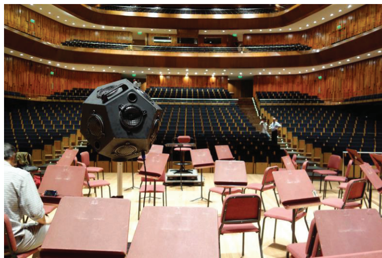
Figure 8: Dodecahedral speaker used in the 2016 measurements (IADAE)
