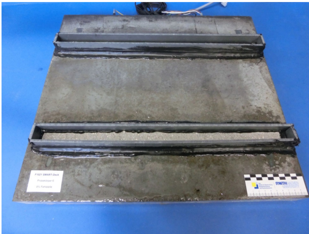
FIGURE 7 Specimen for the detectability-test with two artificial leakages [Color figure can be viewed at wileyonlinelibrary.com ]
