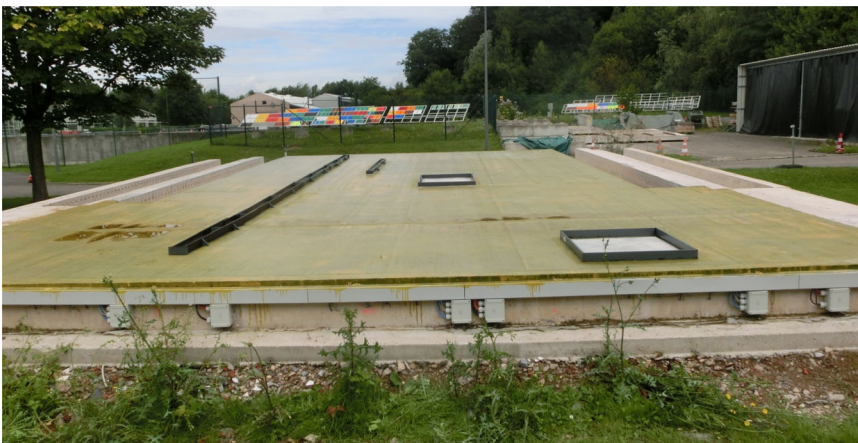
FIGURE 11 Sealed demonstrator with artificial leakages [Color figure can be viewed at wileyonlinelibrary.com ]
