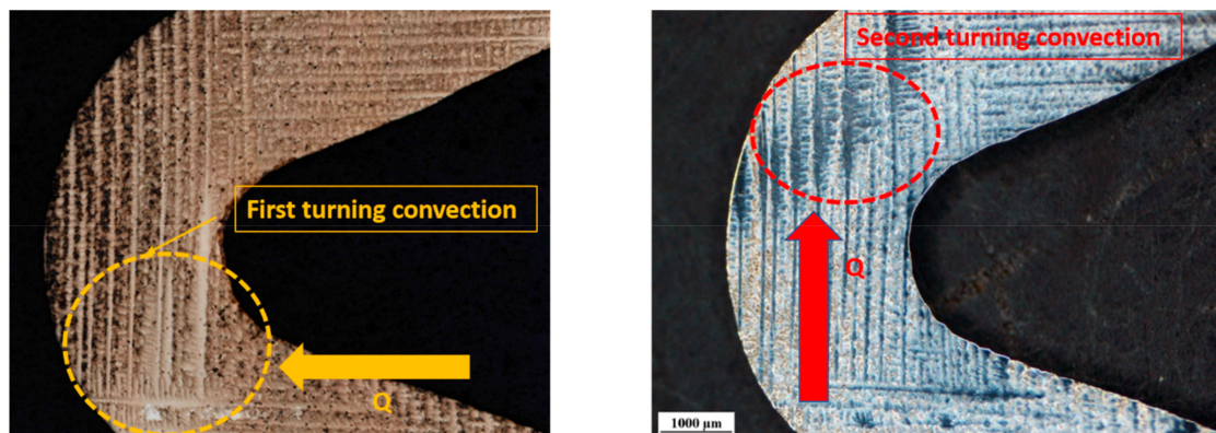
Figure 10. The dendrite turning convection relationship with the heat flow.
