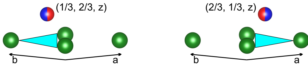
Figure 4.22: Two bottom atomic layers of GST film considered in calculations. Both configurations are energetically equivalent if they are not placed on Si(111) substrate. When they are placed on a Si(111) substrate, they play as a starting point for opposite rotational twin domains. Green balls display Te atoms, and red/blue – Ge/Sb atoms.
