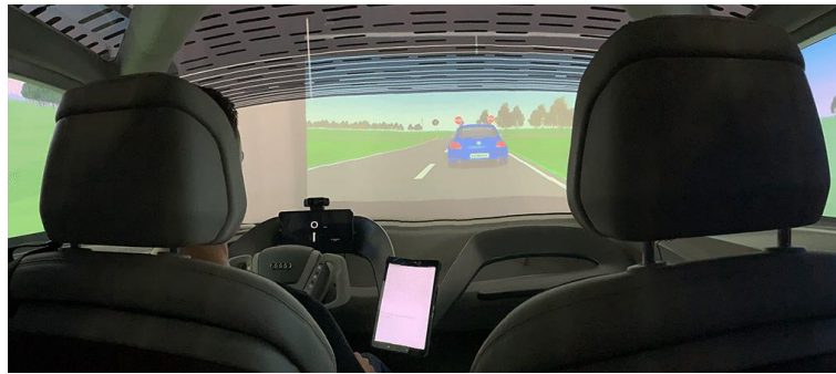
Figure 3.2 AUDI mockup from 2010 combined with external and internal screens for a static driving simulator setup.
