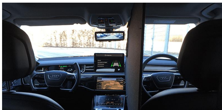
Figure 3.3 Interior view of the Wizard of Oz setup used for real-world driving scenarios (Sauer, Mertens, Reiche et al., 2020).
