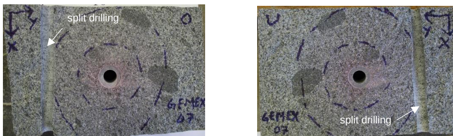
Figure 18: Split plane with coloured and marked fracture zone of Granite 02 (left: top piece, right: bottom piece)
