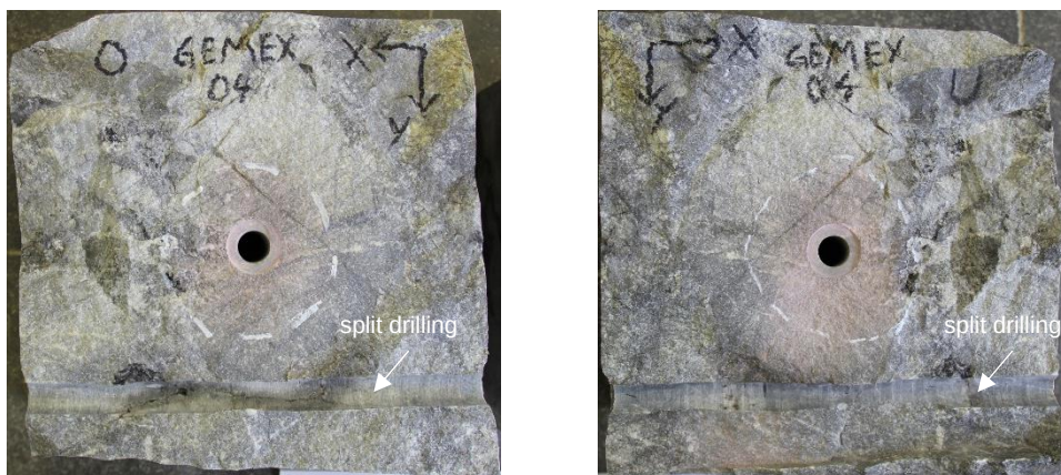
Figure 24: Split plane with coloured and marked fracture zone of Marble 02 (left: top piece, right: bottom piece)
