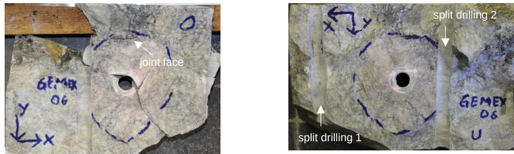
Figure 21: Split plane with coloured and marked fracture zone of Marble 01 (left: top piece, right: bottom piece)
