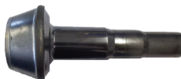
Fig. 8. Preformed and forged parts in production of bevel gear. Dimensions are approximate and in mm.
