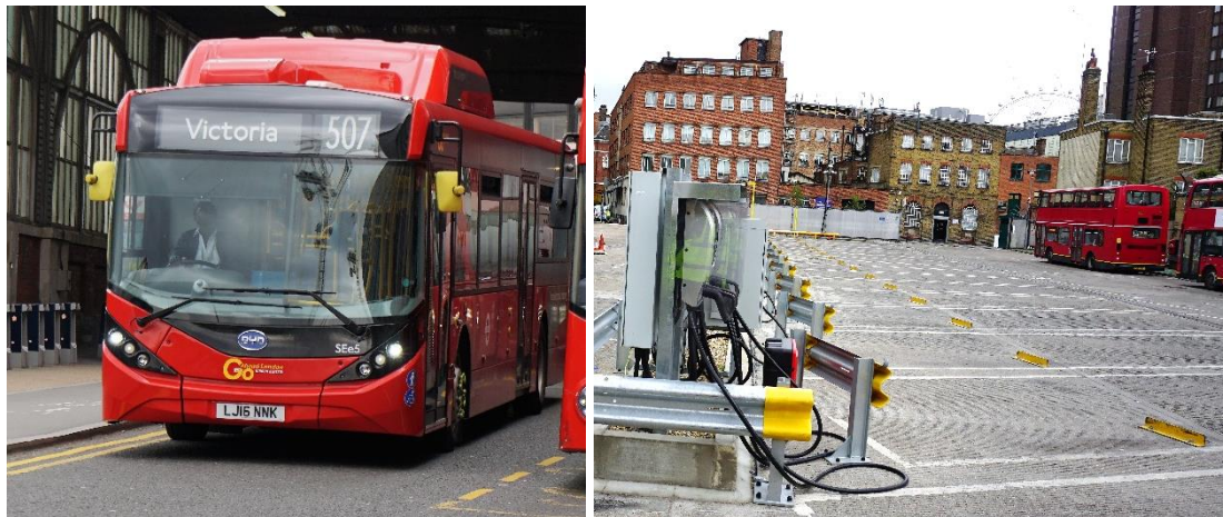
Figure 2-2: BEB Enviro200EV from the manufacturer BYD/ADL (left) and charging infrastructure at the Waterloo depot in central London (right)
