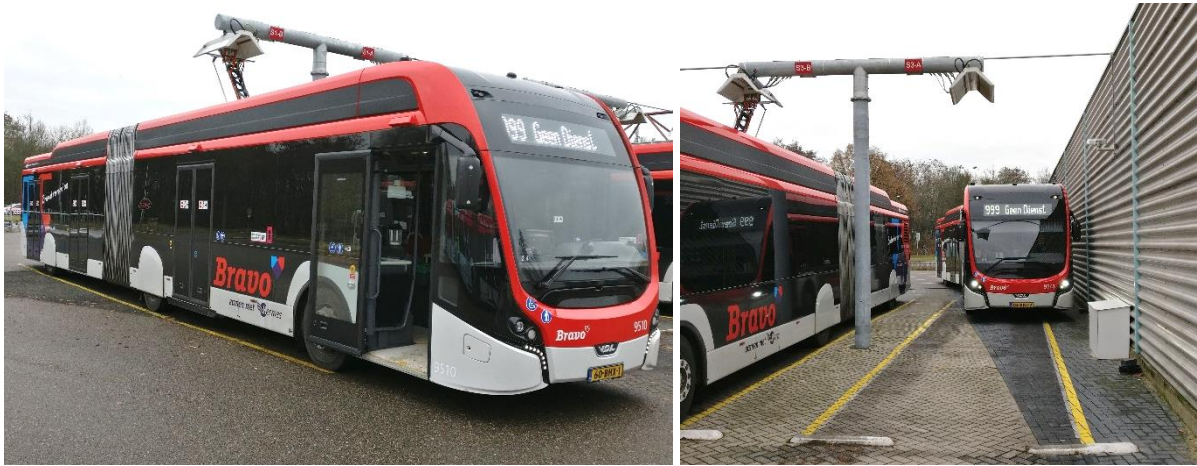
Figure 2-3: BEB Citea SLFA-181 from the manufacturer VDL and charging stations in the Hermes bus depot in Eindhoven (NL)
