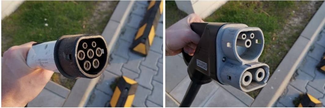
Figure 3-7: Type 2 (AC-charging) and Combo Type 2 (DC-charging) plugs utilized as coupling system for BEB
