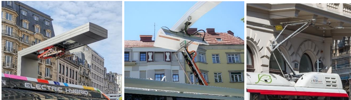
Figure 3-8: Charging pantographs at terminal stops – stationary-mounted inverted pantograph (left), vehicle-mounted pantograph with charging hood (center) and vehicle-mounted pantograph with catenaries 2 (right)
