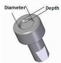
Figure 4.33: The flat die design (88).
