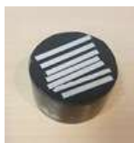
Figure 4.40: An example of a hot mounted sample.
