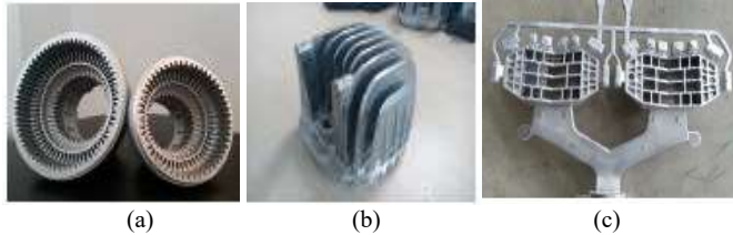
Figure 2.21: (a) Dock cleat (b) LED housing and (c) Brackets for the telecom industry.
