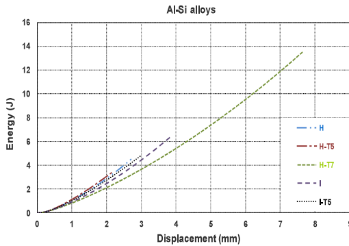
Figure 5.10 : The simulated energy-displacement chart of the Al-Si alloys and alloy-heat treatment combinations. ( Designations from Table 4.3, P54 )
