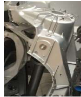
Figure 2.2: Jaguar XE/XF- Front shock tower ( Magna BDW technologies Soest GmbH ).
