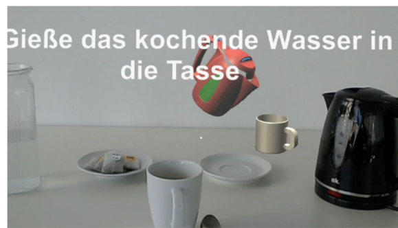
Fig. 1 Display of holographic cues presented by the Therapy Lens application on a Microsoft HoloLens. The subtitle and holograms indicate the first step in the tea making task of pouring the heated water into the mug ("Gieße das kochende Wasser in die Tasse"). The red kettle and the small white mug (on the right) are both holographic objects
