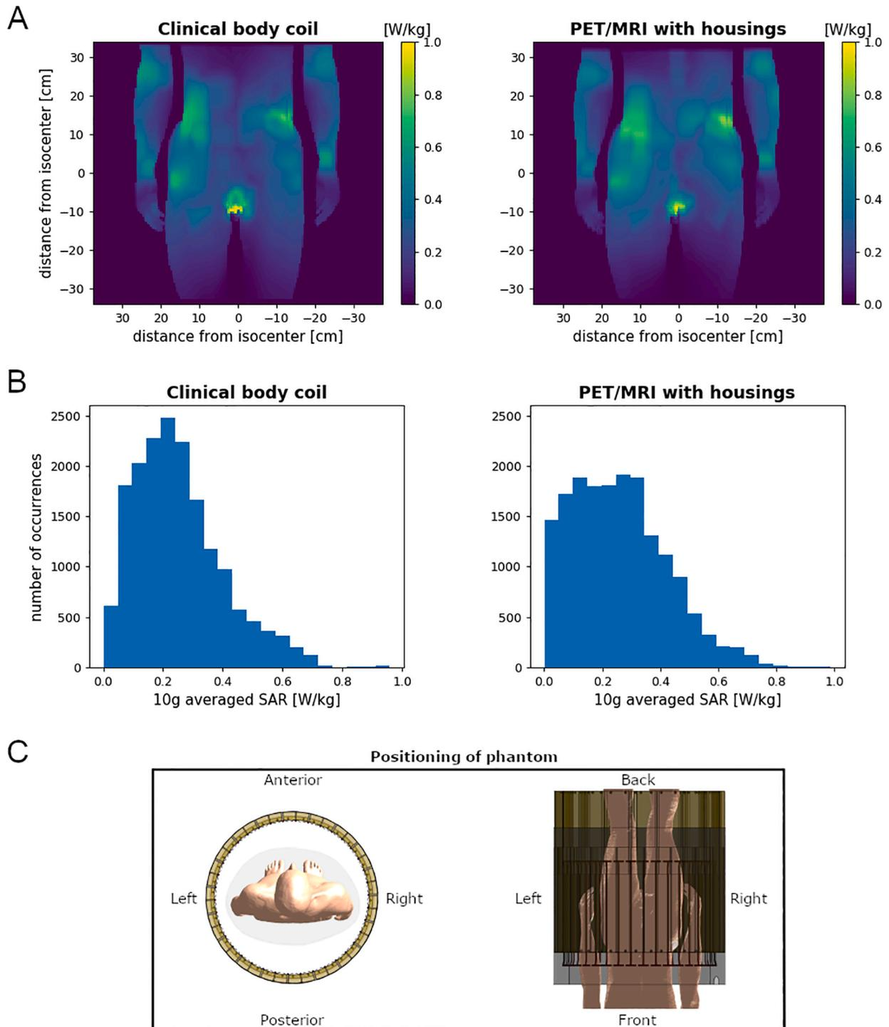
**Fig. 3.** Results of SAR simulations. (A) Maximum intensity plots of 10 g averaged SAR. (B) Histograms of SAR values in all non-zero voxels. (C) Positioning of phantom in PET/MRI body coil during SAR simulations.
