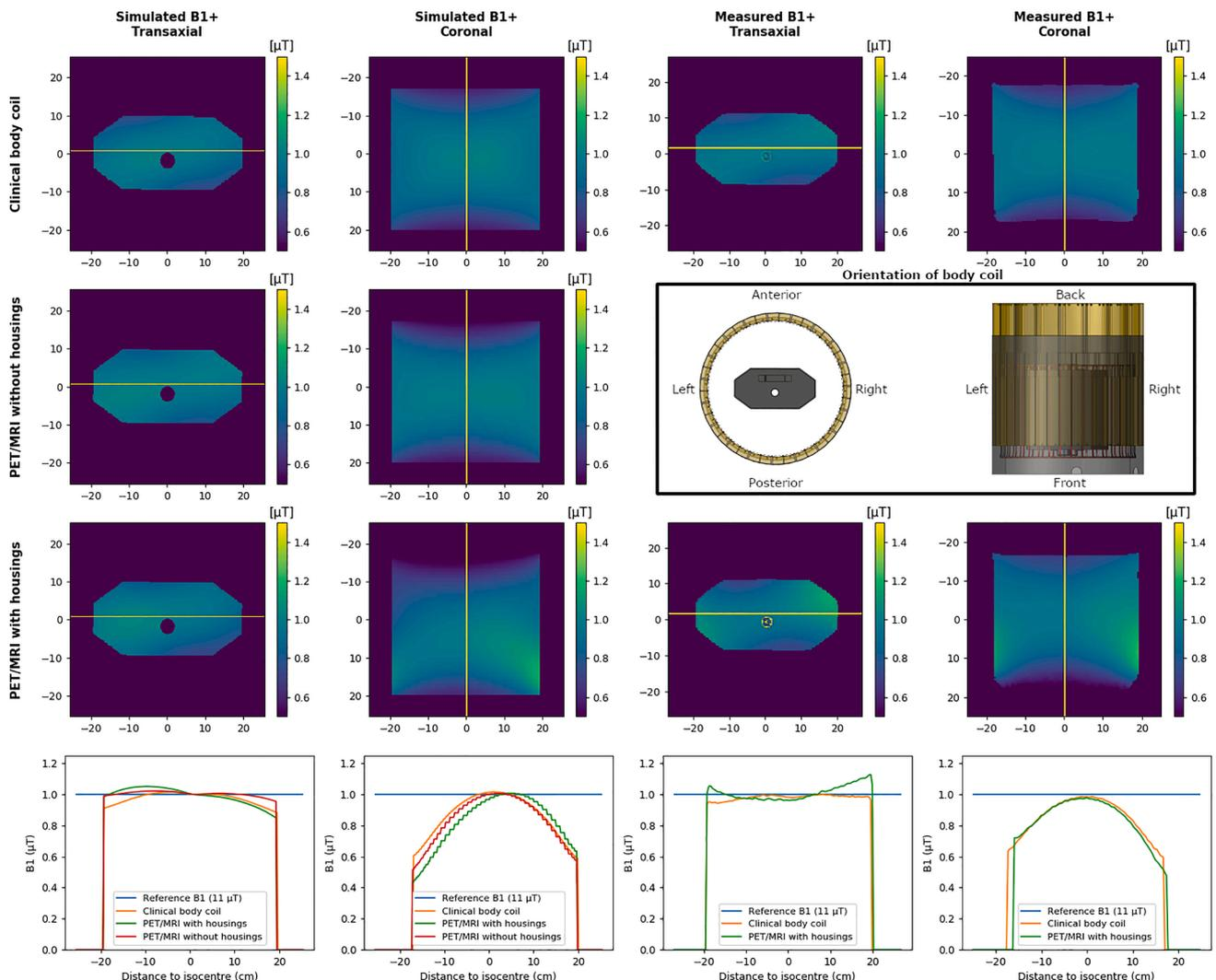
Fig. 2. Simulated and measured  $B_1^+$  transmit field maps (central transaxial and coronal slices) and image profiles. The yellow lines in the  $B_1^+$  maps indicate the locations of the image profiles.
