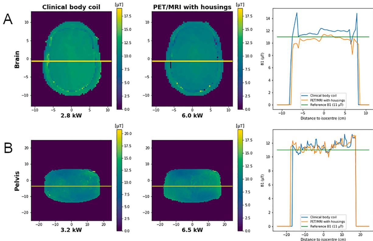
**Fig. 4.**  $B_1^+$  maps and image profiles of volunteer scans. (A) Central transaxial slices through the volunteer’s brain. (B) Central transaxial slices through the volunteer’s pelvis. Yellow lines indicate the locations of the image profiles.
