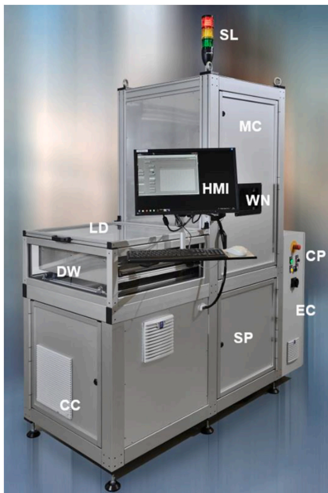
Fig. 8. Scanning LIBS set-up with 2D, 3D geometry measurements. EC electric cabinet with supply for scanner, axes and control electronics; CP control panel; CC control computer, laser cooler, laser power supply; SP multi-CCD spectrometer; LD lid to be opened to load the drawer (translation stage); DW drawer to charge the measuring objects; MC measuring cabinet with 2D, 3D cameras, scanner, laser source; SL signal light; HMI touch screen; WN observation window according to laser safety requirements.
